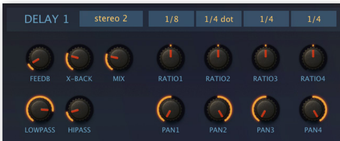
Delay module in 'stereo 2' mode (ping-pong regeneration via x-back)
