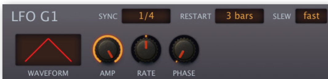
LFOG module, triangle wave, synced to ‘beats’ and retriggered every 3 bars
