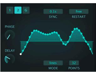
Please note that SYNC (see above) sets the length of each step, so a complete cycle in the lefthand example would take 8 times 1/16 = half a bar in 4/4 time. In the righthand example a complete cycle would take 32 times 0.1 seconds = 3.2 seconds.
