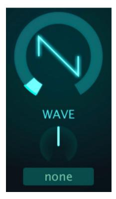
The lower knob is for waveform modulation – click on the label ('none') and select a source. The waves were chosen to (loosely) alternate between 'dull' and 'bright', which is why the maximum modulation depth is 2.00: ZebraCM is not a wavetable synth.
