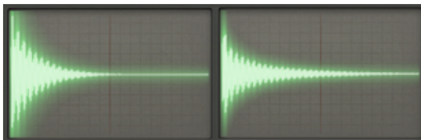
envelope decays with Snappy switched off (L), and switched on (R)
